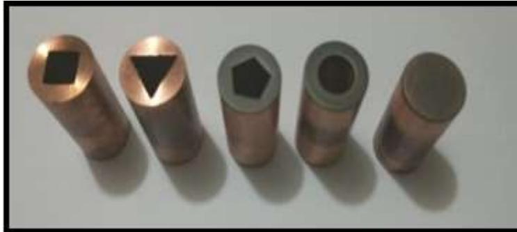
Fig. (5): four hollow shape and solid of copper electrode.
